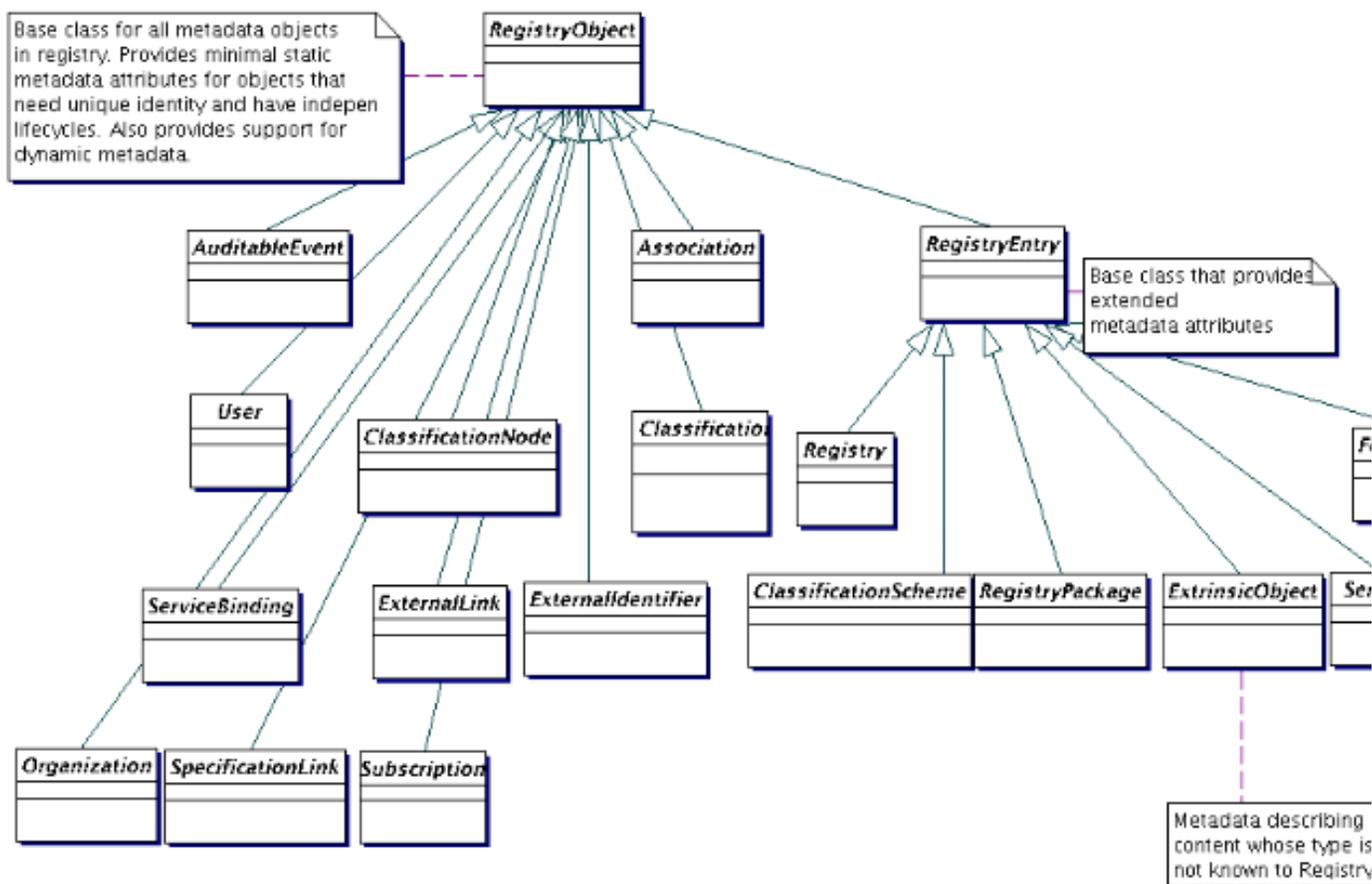
**Figure 5: ebXML Registry Information Model: Inheritance View"**
